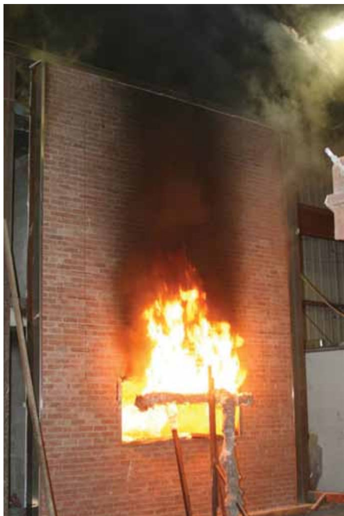
Figure 2. An NFPA 285 test in progress.
