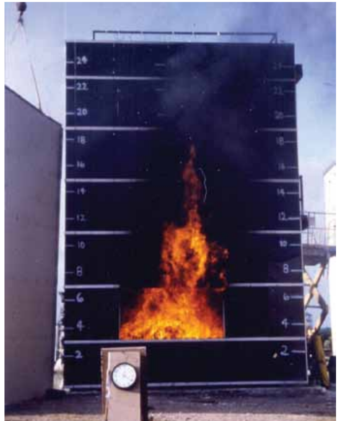
Figure 1. UBC 17-6 test in progress.
