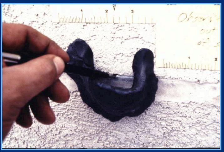
Not a standard ASTM or AAMA test; putty, modeling clay, Duxseal or Dow Dilatant Putty.
