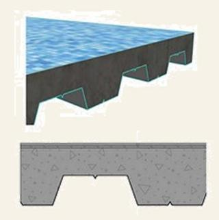
Steel decking has a high rate of thermal transmission and does not adversely impact the energy transfer.
